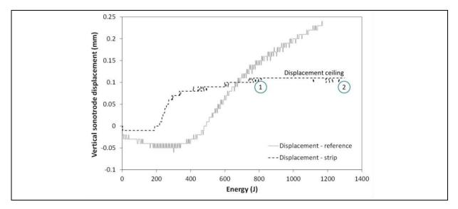
**Figure 2:** Comparison between displacement curves of a regular single lap shear weld with ED covering the entire overlap area (reference, [1]) and a 25 mm overlap with an ED strip (as shown in Figure 1 (b)). Circled numbers show the two stages where the welding process was stopped to investigate changes in the fracture surfaces.
