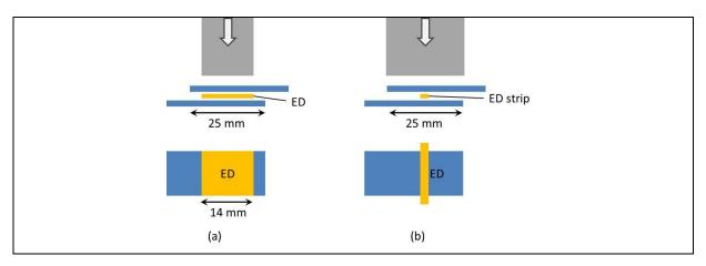
Figure 1: (a) 25 mm overlap and energy director with the same width as sonotrode (14 mm) [2], and (b) ED strip in a 25 mm overlap with sonotrode covering the entire overlap. Dimensions are not to scale.
